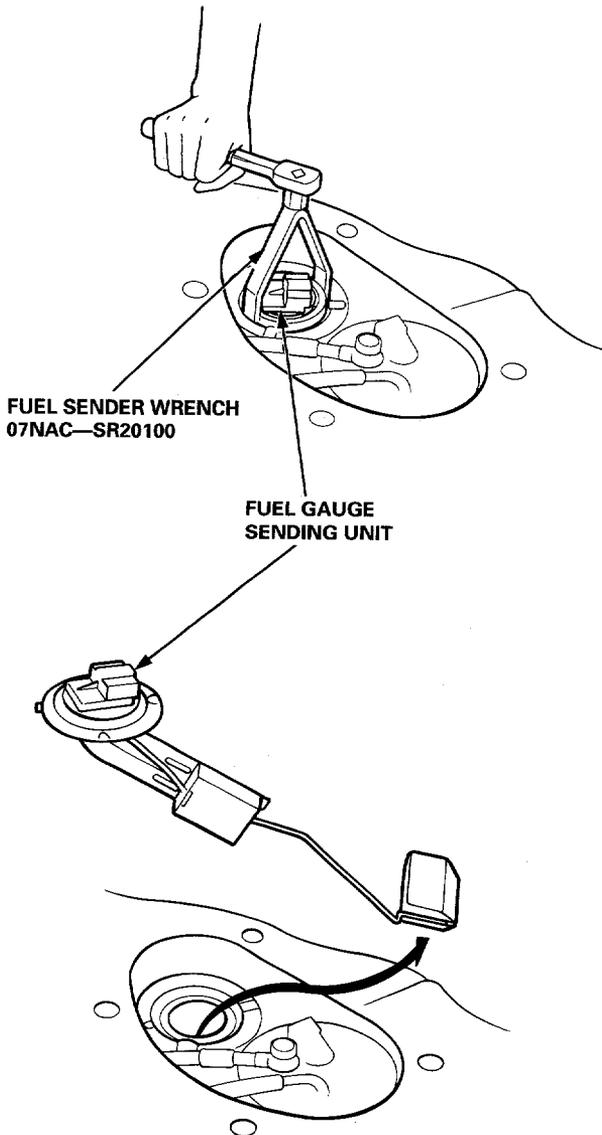
4. Measure the resistance between the B and C terminals at E (EMPTY), 1/2 (HALF FULL) and F (FULL) by moving the float.
